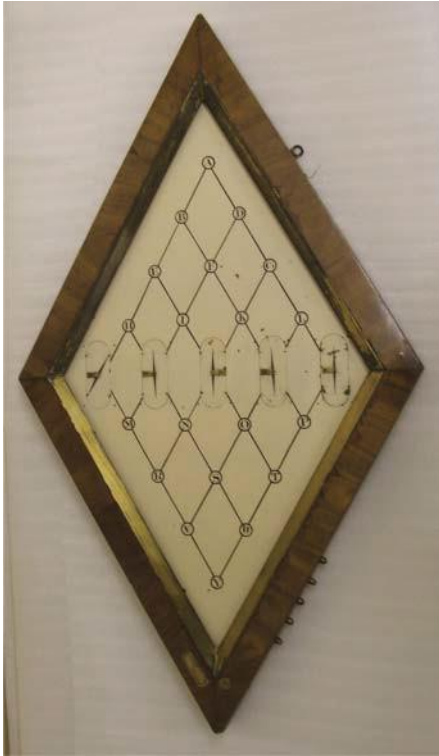
figure 5 Large five-needle Cooke and Wheatstone electric telegraph dial with individual needle mountings, probably one of the instruments demonstrated at Euston and Camden Town in 1837. On loan to National Museums Scotland from King's College London. NMS T.1951.L23.
