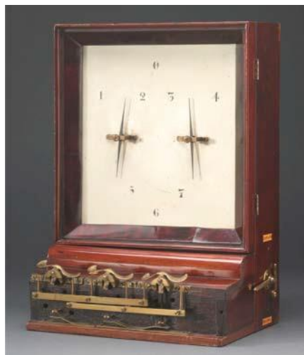
figure 8 W. F. Cooke's double-needle portable telegraph instrument of 1838, fitted with Cooke's centrally pivoted operating keys ('Heidelberg keys'). ScM Inv. 2004-105, ScM/SSPL 10459328.
