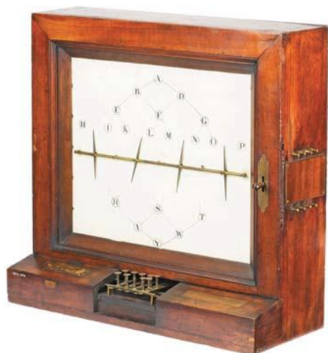
figure 7 A prototype, fitted with Wheatstone's ten-button permutating keyboard, of the four-needle electric telegraph instruments patented by W. F. Cooke in 1838 and installed on the Great Western Railway between Paddington and West Drayton in 1839. ScM Inv. 1876-1274, ScM Photo Studio 1876-1274_ (0001).
